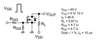
Fig. 6.2.1 Switching Time Test Circuit
