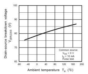
Fig. 8.7 V<sub>(BR)DSS</sub> - T<sub>a</sub>
