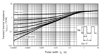
Fig. 8.13 r<sub>th</sub> - t<sub>w</sub> (Guaranteed Maximum)
