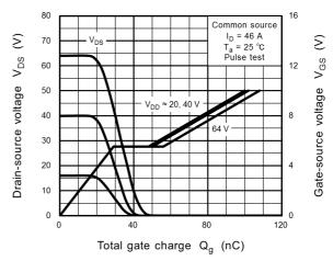
Fig. 8.10 Dynamic Input/Output Characteristics
