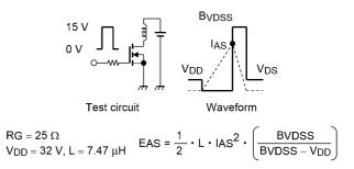
Fig. 8.16 Test Circuit/Waveform
