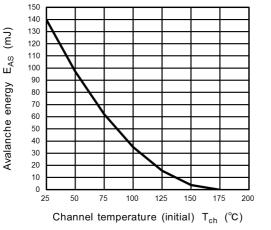
Fig. 8.15 E<sub>AS</sub> - T<sub>ch</sub>(Guaranteed Maximum)
