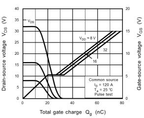
Fig. 8.14 Dynamic Input/Output Characteristics
