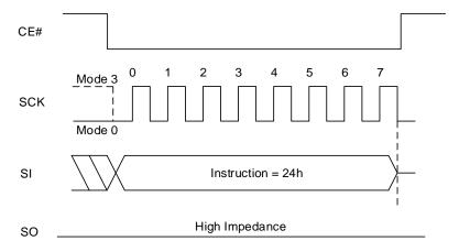
Figure 8.69 Sector Lock Sequence In QPI Mode
