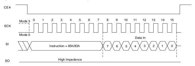
Figure 8.40 Set Extended Read Parameters Sequence In QPI Mode
