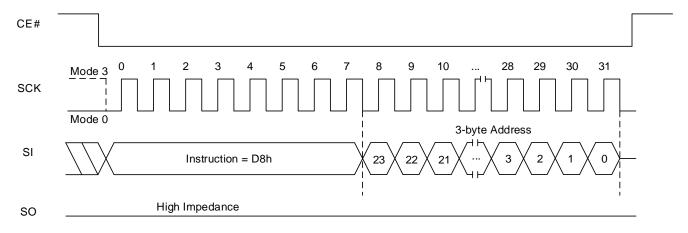
Figure 8.16 Block Erase (64K) Sequence In QPI Mode (D8h)
