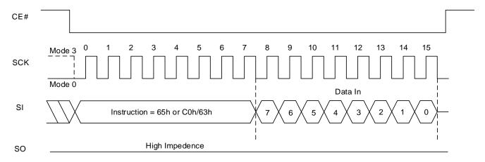
Figure 8.38 Set Read Parameters Sequence In QPI Mode
