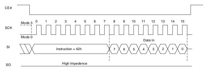
Figure 8.30 Write Function Register Sequence In QPI Mode
