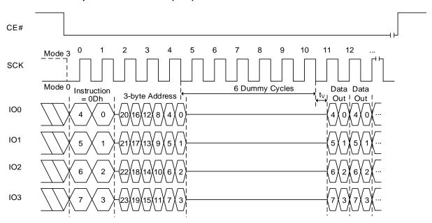
Figure 8.61 FRDTR Sequence In QPI Mode (0Dh)
