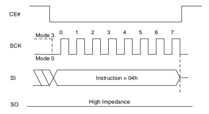
Figure 8.22 Write Disable Sequence In QPI Mode
