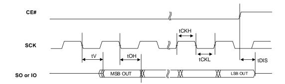
Figure 9. 5 OUTPUT TIMING (DTR Mode)
