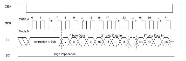
Figure 8.97 Unlock Password Sequence In SPI Mode
