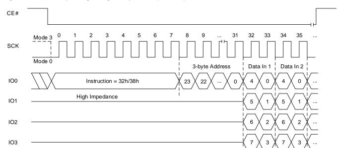
Figure 8.12 Quad Input Page Program operation (32h/38h)
