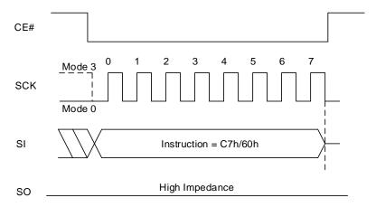
Figure 8.18 Chip Erase Sequence In QPI Mode
