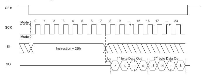
Figure 8.85 Read ASP Sequence In QPI Mode
