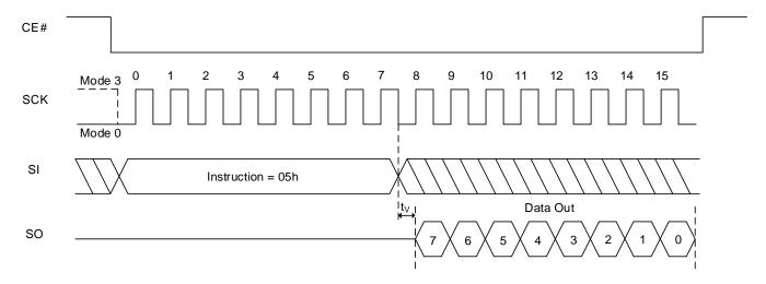
Figure 8.24 Read Status Register Sequence In QPI Mode
