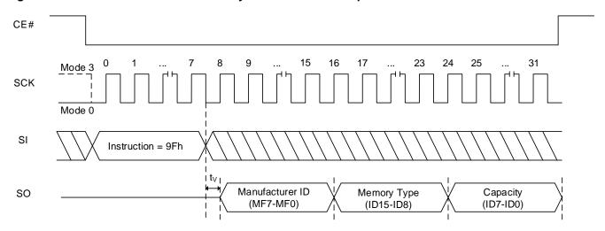
Figure 8.50 RDJDID and RDJDIDQ (Read JEDEC ID) Sequence In QPI MOde
