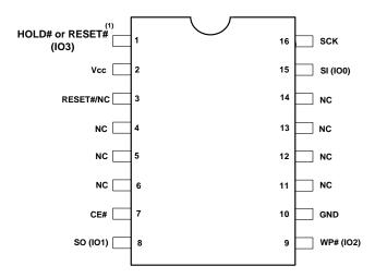
16-pin SOIC 300mil (Package: M)
