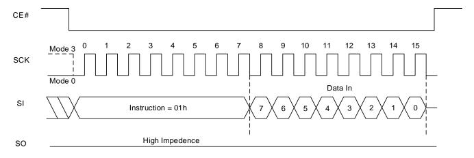
Figure 8.26 Write Status Register Sequence In QPI Mode
