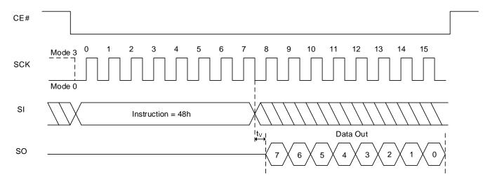
Figure 8.28 Read Function Register Sequence In QPI Mode
