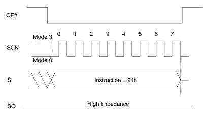
Figure 8.92 Set FREEZE Bit Sequence In QPI Mode
