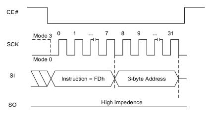
Figure 8.81 Program PPB Sequence In QPI Mode (FDh)
