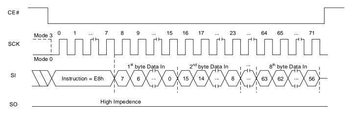
Figure 8.95 Program Password Sequence In QPI Mode
