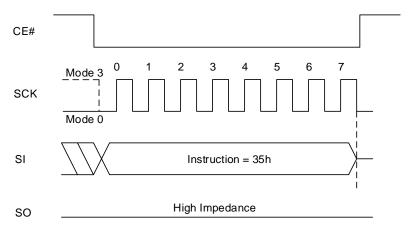
Figure 8.32 Exit Quad Peripheral Interface (QPI) Mode Sequence
