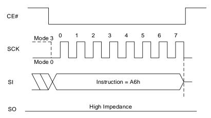
Figure 8.90 Write PPB Lock Bit Sequence In QPI Mode
