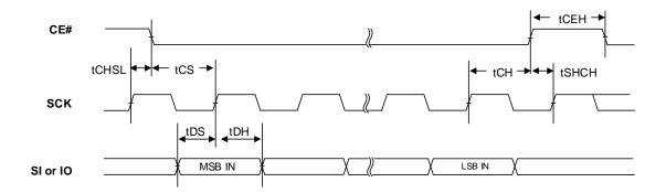
Figure 9.3 SERIAL INPUT TIMING (DTR Mode)
