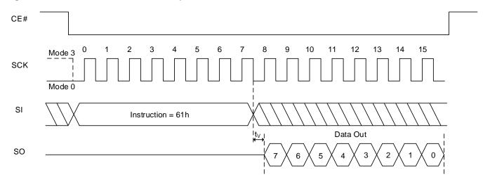
Figure 8.42 Read Read Parameters Sequence In QPI Mode
