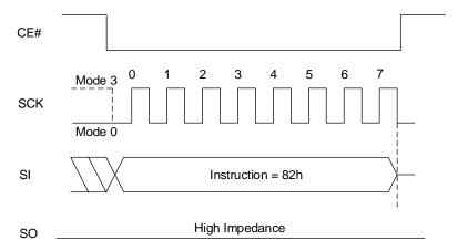
Figure 8.46 Clear Extended Read Register Sequence In QPI Mode
