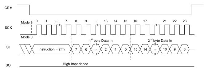
Figure 8.87 Program ASP Sequence In QPI Mode
