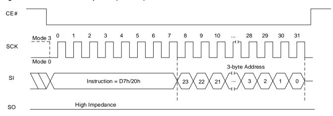
Figure 8.14 Sector Erase Sequence In QPI Mode (D7h/20h)
