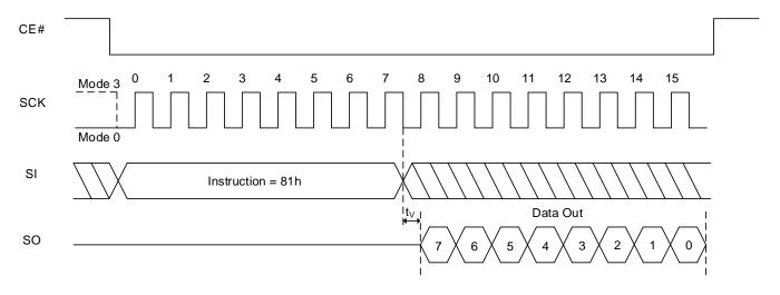
Figure 8.44 Read Extended Read Parameters Sequence In QPI Mode
