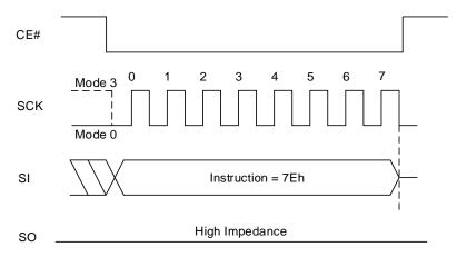
Figure 8.99 Gang Sector/Block Lock Sequence In QPI Mode
