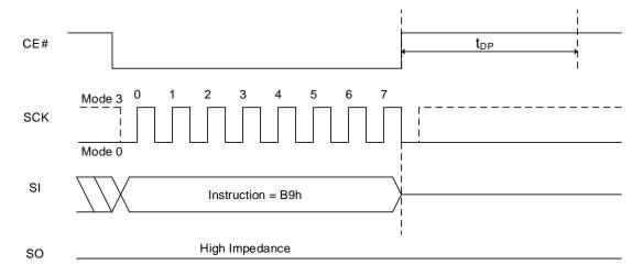
Figure 8.34 Enter Deep Power Down Mode QPI Sequence
