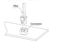
Insert the pilot into the connector, as shown in.
