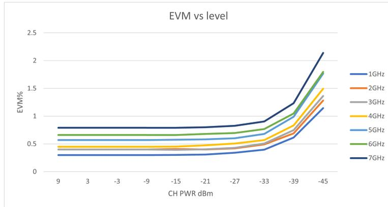
For RSA5100B Series Spectrum Analyzers:  $\leq 44.4$  dB rms EVM from 1 GHz to 7 GHz
