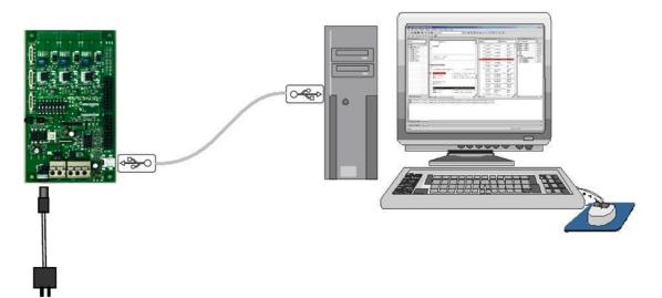
Figure 1: RL78/I1A DC/DC LED Control Evaluation Board System Configuration
