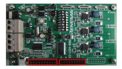
Figure 5: External Connectors J1 and J2
