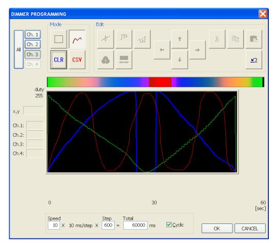
Figure 43: Applilet EZ for HCD Controller Wave Editor (3 channels)
