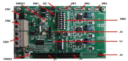
Figure 2: RL78/I1A DC/DC LED Control Evaluation Board Components
