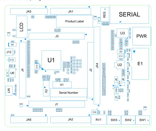
Figure 3-3: Top-Side Component Placement
