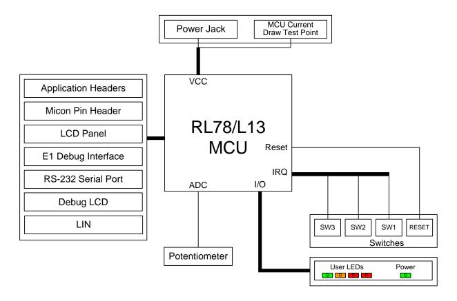
Figure 4-1: Internal RSK Block Diagram
