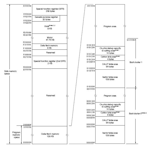
**Notes 1.** Use of the area FFE20H to FFEDFH and FDF00H to FE309H is prohibited when using the self-programming function and data flash function, because this area is used for self-programming library.
