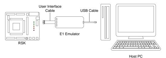
Figure 4-2: Debugger Connection Diagram
