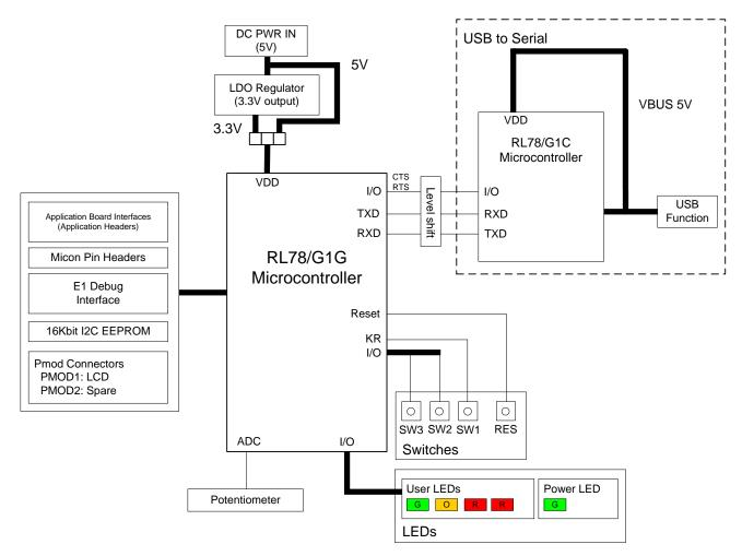
Figure 4-1: Internal RSK Block Diagram
