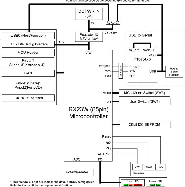
In addition to DC PWR IN, VBUS (USB0 Function / USB to Serial Function) can be used as the power supply source for the board.
