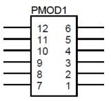
Figure 5-1: Digilent Pmod<sup>™</sup> Compatible Header Pin Numbering
