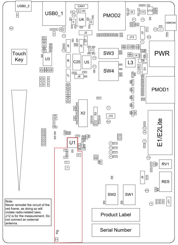
Figure 3-3: Top-Side Component Placement
