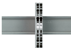
Fuse terminal blocks with a width of 6.2 mm/0.244 in can be assembled adjacently. If there is no adjacent fuse terminal block at the end of the assembly, an end plate must be used.
