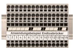
Continuous jumpers (2002 Series) readily connect an endless number of terminal blocks to each other via single jumper slot. Use the second jumper slot for additional commoning or testing.
