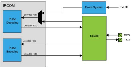
The USART is set in IRCOM mode by writing  $0 \times 02$  to the CMODE bit field in the USARTn.CTRLC register. The data on the TXD/RXD pins are the inverted values of the transmitted/received infrared pulse. It is also possible to select an event channel from the Event System as an input for the IRCOM receiver. This enables the IRCOM to receive input from the I/O pins or sources other than the corresponding RXD pin, which will disable the RxD input from the USART pin.
