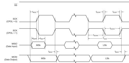
Figure 35-4. SPI - Timing Requirements in Host Mode
