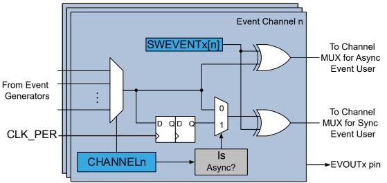
Figure 16-1. EVSYS Block Diagram
