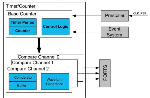
Figure 22-1. 16-Bit Timer/Counter and Closely Related Peripherals
