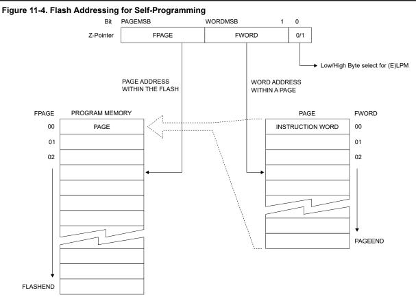
The Flash is word-accessed and organized in pages, so the Address Pointer can be treated as having two sections, as shown in the figure above. The word address in the page (FWORD) is held by the Least Significant bits (LSb) in the Address Pointer, while the Most Significant bits (MSb) in the Address Pointer hold the Flash page address (FPAGE). Together, FWORD and FPAGE hold an absolute address to a word in the Flash.
