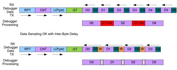
Too Fast Transmission, no Inter-Byte Delay
