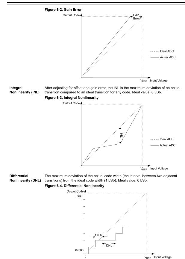
**Quantization Error** Due to the quantization of the input voltage into a finite number of codes, a range of input voltages (1 LSb wide) will code to the same value. Always ±0.5 LSb.
