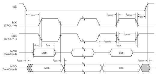
Table 35-20. SPI - Timing Specifications in Client Mode
