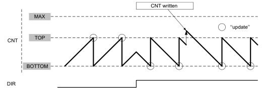
It is possible to change the counter value in the Counter (TCAn.CNT) register when the counter is running. The write access to TCAn.CNT register has higher priority than count, clear or reload, and will be immediate. The direction of the counter can also be changed during ordinary operation by writing to the Direction (DIR) bit in the Control E (TCAn.CTRLE) register.
