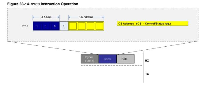
Figure 33-14 shows the data frame transmitted after the SYNCH character and the instruction frames. The STCS instruction byte can immediately be followed by the data byte. There is no response generated from the STCS instruction, as is the case for the ST and STS instructions.
