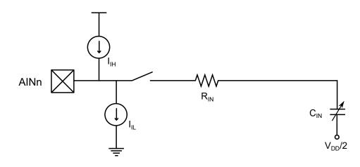
If a source with high impedance is used, the sampling time may need to be increased. The required sample time will depend on how long the source needs to charge the  $C_{IN}$  capacitor and can be configured using the Sample Duration (SAMPDUR) bit field in the Control E (ADCn.CTRLE) register.
