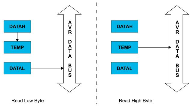
For a 16-bit read operation, the low byte register (e.g., DATAL) of the 16-bit register must be read before the high byte register (e.g., DATAH). When the low byte register is read, the high byte register of the 16-bit register is copied into the temporary (TEMP) register in the same clock cycle, as shown on the left side of the figure above. Reading
