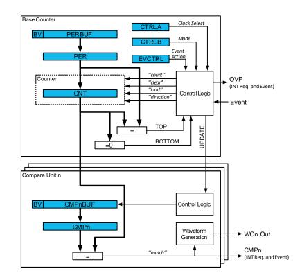
The Counter (TCAn.CNT) register, Period and Compare (TCAn.PER and TCAn.CMPn) registers, and their corresponding buffer registers (TCAn.PERBUF and TCAn.CMPnBUF) are 16-bit registers. All buffer registers have a Buffer Valid (BV) flag indicating when the buffer contains a new value.
