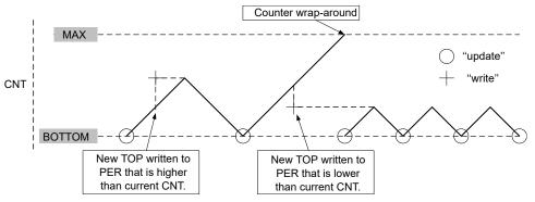
**With Buffering:** When using double-buffering, the buffer can be written at any time and still maintain the correct operation. TCAn.PER is always updated on the UPDATE condition, as shown for dual-slope operation in the figure below. This prevents wrap-around and the generation of odd waveforms.
