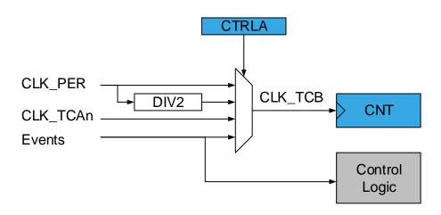
The Clock Select (CLKSEL) bit field in the Control A (TCBn.CTRLA) register selects one of the prescaler outputs directly, or an event channel as the clock (CLK\_TCB) input.
