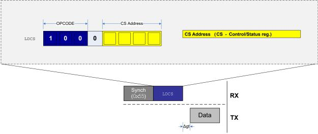
Figure 33-13 shows a typical example of LDCS data transmission. A data byte from the LDCS is transmitted from the UPDI after the guard time is completed.
