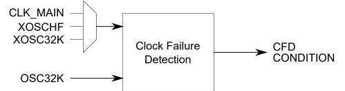
When the CFD feature is enabled, it will monitor the selected source from the Clock Failure Detection Source (CFDSRC) bit field in the Main Clock Control C (CLKCTRL.MCLKCTRLC) register. In sleep, the CFD will only be enabled if the selected source is active.
