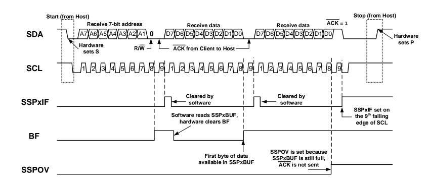
Figure 29-15. I<sup>2</sup>C Client, 7-Bit Address, Reception (SEN = 0, AHEN = 0, DHEN = 0)
