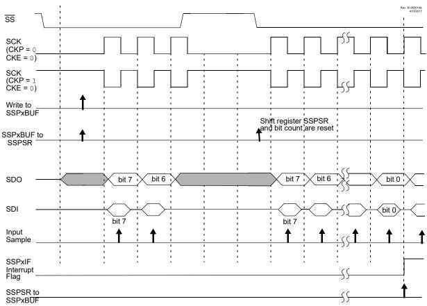
Figure 29-6. Client Select Synchronous Waveform
