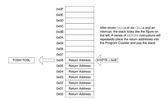
Figure 9-17. Accessing the Stack Example 4
