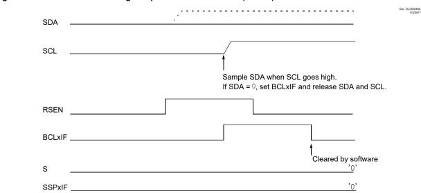
Figure 29-37. Bus Collision During a Repeated Start Condition (Case 1)
