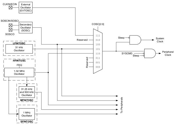
Figure 11-1. Clock Source Block Diagram
