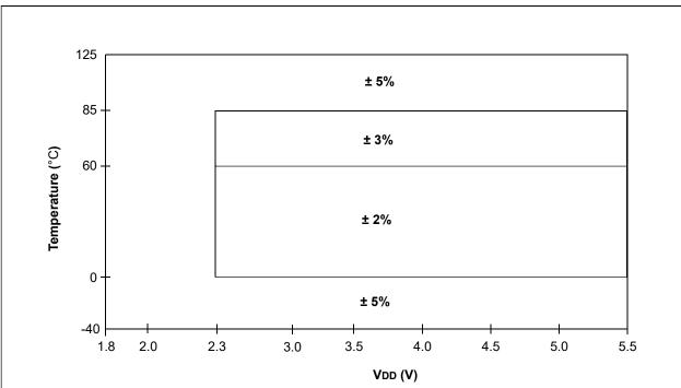
Figure 41-5. Precision Calibrated HFINTOSC Frequency Accuracy Over Device V<sub>DD</sub> and Temperature
