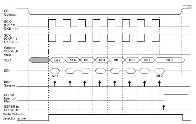
Figure 29-7. SPI Mode Waveform (Client Mode with CKE = 0)
