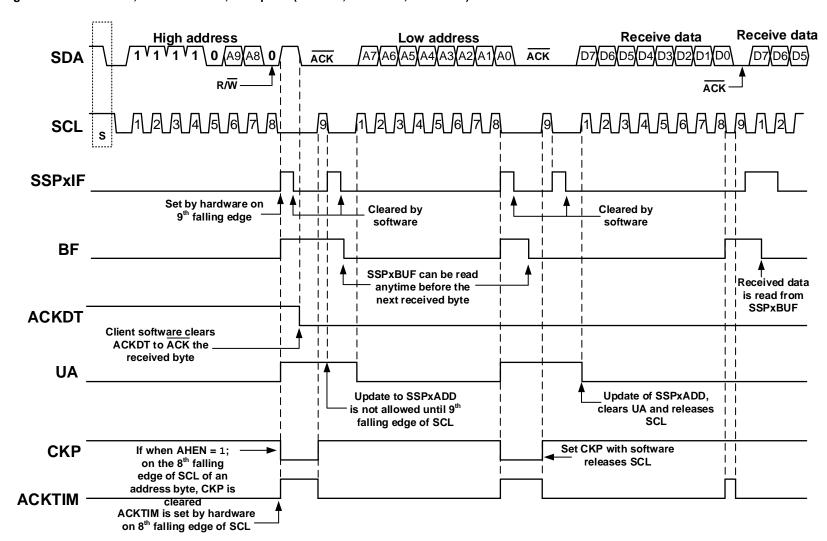
Figure 29-20. I<sup>2</sup>C Client, 10-Bit Address, Reception (SEN = 0, AHEN = 1, DHEN = 0)
