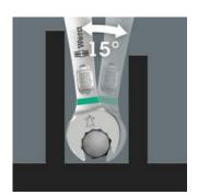
The Joker 6005 double openended wrench with its special mouth design - a 7.5° pivoted mouth and double hexagon geometry - doubles the placement points at a repeated 180° rotation of the wrench around the longitudinal axis. Bolts and screw heads can be engaged every 15°. The Joker 6005 will automatically find the respective placement point after every turn.
