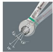
the pivoted Thanks to 7.5° mouths, the double hexagon geometry and an improved application method (placement screwdriving - rotation - replacement - screwdriving - rotation etc), even screwdriving situations that have a pivoting angle of less than 30° can be solved.
