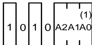
Figure 44. Difference of Slave Address of Each Type
