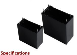
Type 953B radial leaded metallized polypropyene capacitors are designed for UPS systems and other AC output filtering applications. With an integrated fused metallization pattern, this product features UL 810 recognition for fail-safe operation at temperatures up to 85 °C while meeting THB 85 °C / 85% RH testing at rated voltage for challenging harsh environments.
