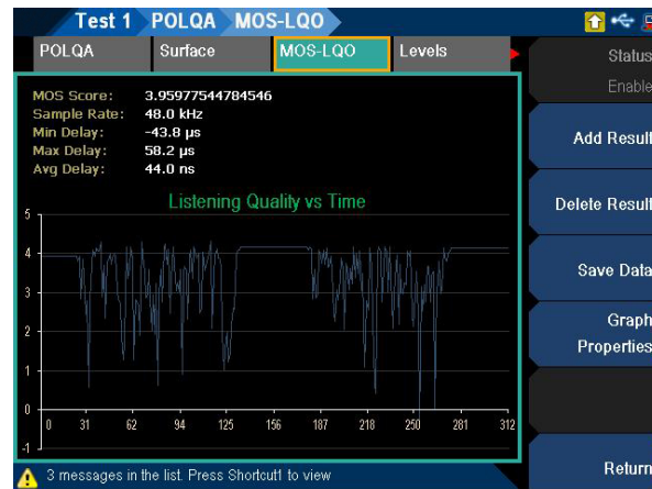
Figure 8. The MOS (Mean Opinion Score) scoring, indicating the rating of the DUT's voice quality.
