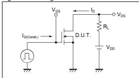
Fig.3-1 Avalanche Measurement Circuit
