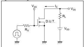
Fig.2-1 Gate Charge Measurement Circuit
