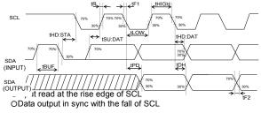
Figure 1.-(a). Serial Input / Output Timing
