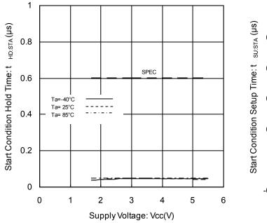
Figure 16. Start Condition Hold Time vs Supply Voltage
