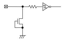
Figure 49. Input Pin Circuit Diagram
