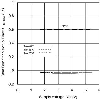
Figure 17. Start Condition Setup Time vs Supply Voltage
