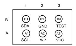
Figure 3. Pin Configuration (BOTTOM VIEW)
