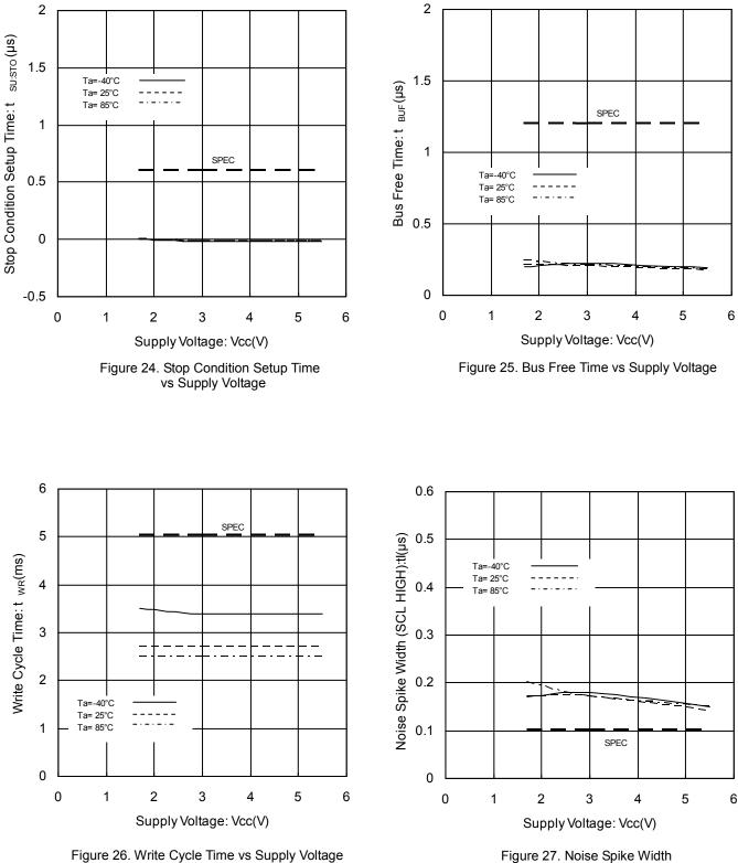
Figure 27. Noise Spike Width vs Supply Voltage (SCL HIGH)
