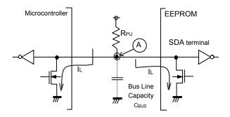
Figure 44. I/O Circuit Diagram
