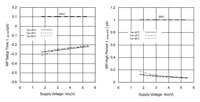
Figure 32. WP Setup Time vs Supply Voltage
