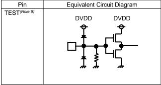
(Note 9) Short the TEST pin to DVSS.
