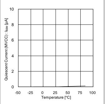
Figure 4. Quiescent Current (MVCC) vs Temperature
