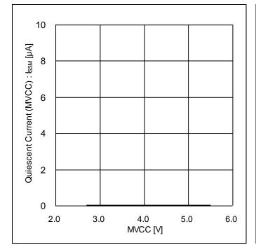
Figure 3. Quiescent Current (MVCC) vs MVCC
