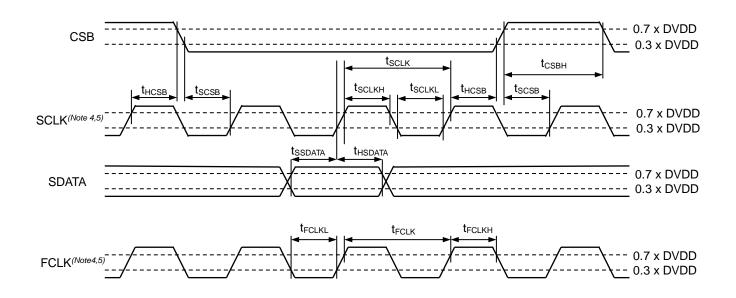
(Note 4) FCLK is asynchronous with SCLK. (Note 5) The duty of FCLK and SCLK is arbitrary after observing the above table.
