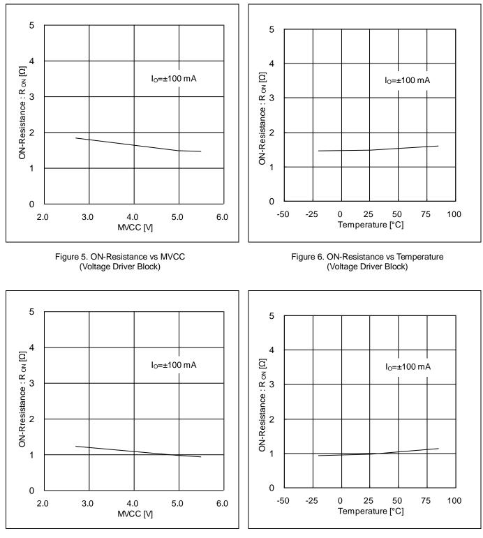
Figure 8. ON-Resistance vs Temperature (Current Driver Block)
