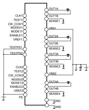
Figure 1. BD63888AEKV Application Circuit Diagram
