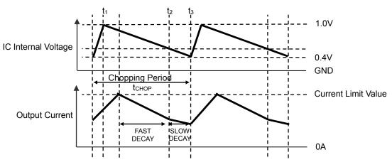
Figure 6. Internal Voltage and Output Current during MIX DECAY
