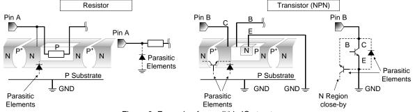
Figure 9. Example of monolithic IC structure
