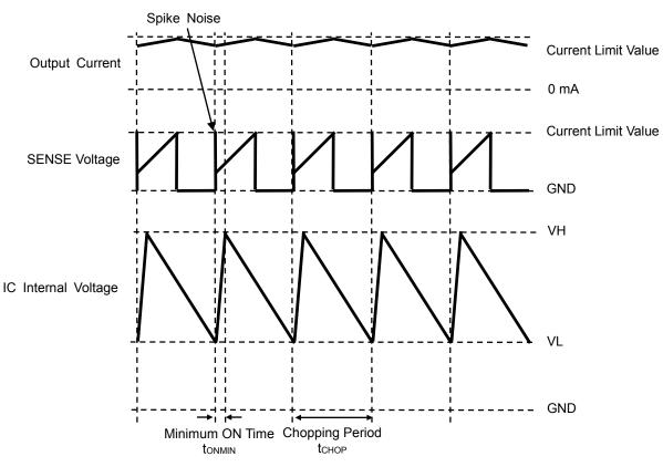
Figure 4. Timing Chart of IC Internal Voltage, the SENSE pin voltage and Output Current
