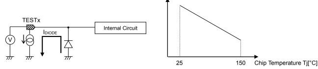
Figure 7. Model Diagram for Measuring Chip Temperature
