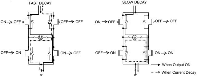
Figure 5. Route of Regenerated Current during Current Decay
