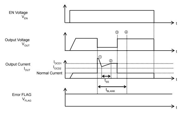
Figure 39. The timing chart without Latch-off when IOUT after Fixed Overcurrent Limit (IOCD1) detection is equal to IOCD2 or higher
