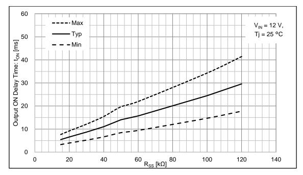
Figure 44. Output ON Delay Time vs R<sub>SS</sub> (V<sub>IN</sub> = 12 V, Tj = 25 °C)
