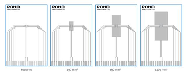
Figure 2. PCB Layout 1 Layer (1s)
