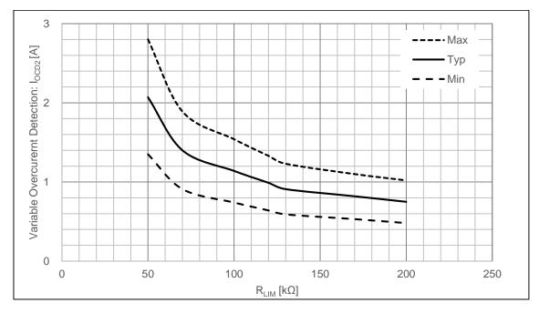
Figure 43. Variable Overcurrent Detection vs RLIM
