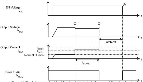
Figure 41. The timing chart of Latch-off function due to Variable Overcurrent Detection (I<sub>OCD2</sub>)
