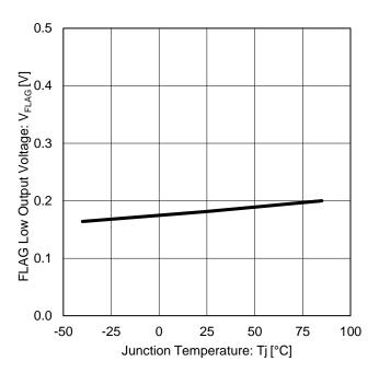
Figure 24. FLAG Low Output Voltage vs Junction Temperature
