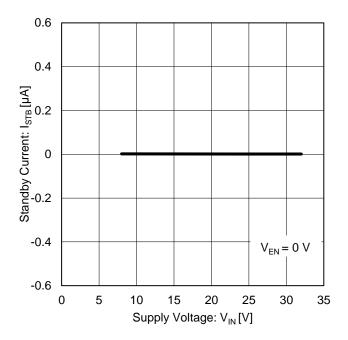
Figure 7. Standby Current vs Supply Voltage
