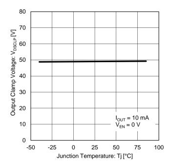
Figure 23. Output Clamp Voltage vs Junction Temperature
