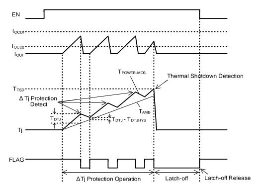
Figure 48. Timing chart of thermal shutdown function and ΔTj protection function with Latch-off function
