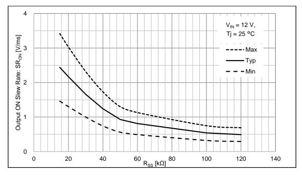
Figure 46. Output ON Slew Rate vs R<sub>SS</sub> ( $V_{IN}$  = 12 V, Tj = 25 °C)
