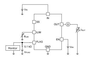
Figure 35. Fixed Overcurrent Limit Variable Overcurrent Detection
