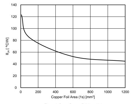
Figure 6.  $\theta_{JA}$  vs Copper Foil Area (1s)
