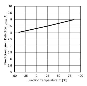
Figure 26. Fixed Overcurrent Limit vs Junction Temperature
