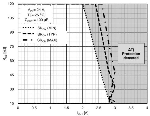
Figure 52.  $\Delta$ Tj protection function detection region at startup (V<sub>IN</sub> = 24 V, C<sub>OUT</sub> = 100  $\mu$ F)
