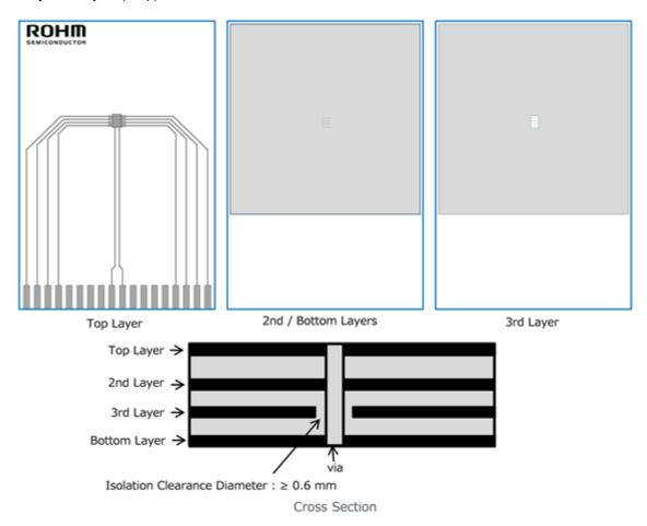
Figure 4. PCB Layout 4 Layers (2s2p)
