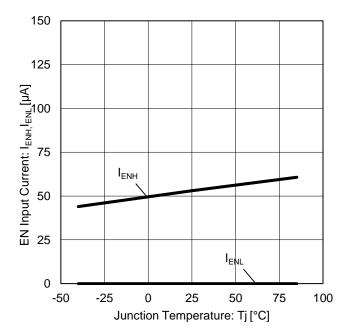
Figure 14. EN Input Current vs Junction Temperature
