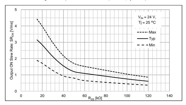
Figure 47. Output ON Slew Rate vs R<sub>SS</sub> ( $V_{IN}$  = 24 V, Tj = 25 °C)
