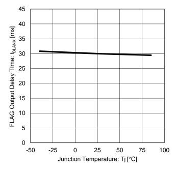
Figure 25. FLAG Output Delay Time vs Junction Temperature
