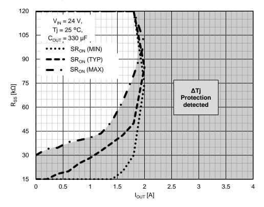
Figure 54.  $\Delta$ Tj protection function detection region at startup ( $V_{IN}$  = 24 V,  $C_{OUT}$  = 330  $\mu$ F)
