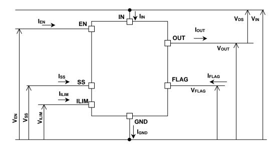
Figure 1. Voltage and Current Definition
