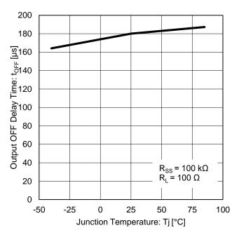
Figure 22. Output OFF Delay Time vs Junction Temperature
