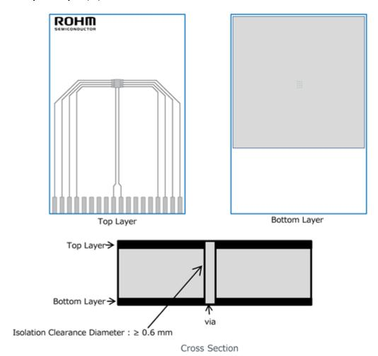
Figure 3. PCB Layout 2 Layers (2s)
