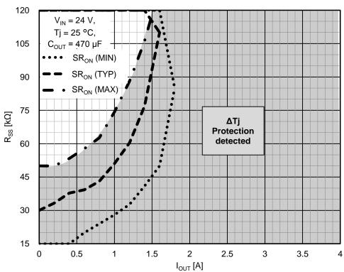
Figure 55.  $\Delta$ Tj protection function detection region at startup ( $V_{IN}$  = 24 V,  $C_{OUT}$  = 470  $\mu$ F)
