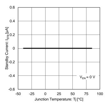
Figure 8. Standby Current vs Junction Temperature
