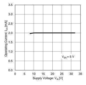
Figure 9. Operating Current vs Supply Voltage
