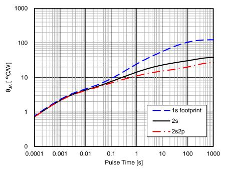
Figure 5.  $\theta_{JA}$  vs Pulse Time
