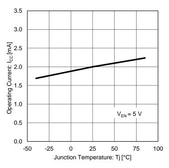
Figure 10. Operating Current vs Junction Temperature
