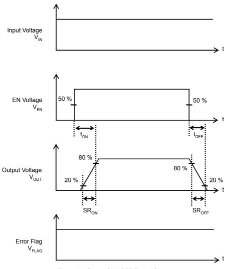
Figure 36. Output ON / OFF Timing Chart
