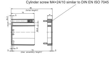
\*\* Dimension reduced at bottom due to conical form. Tolerances to DIN 16901-130
