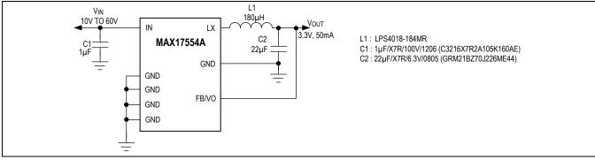
Figure 3. Fixed 3.3V, 50mA Step-Down Converter Output with 10V VINMIN
