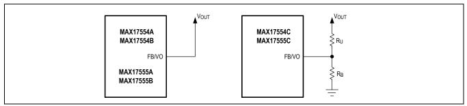
Figure 2. Setting the Output Voltage
