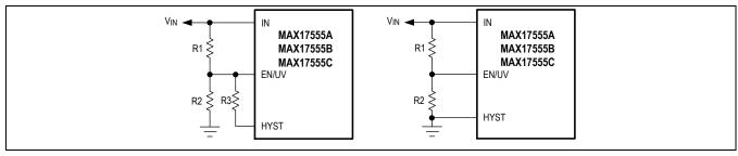
Figure 1. Setting the Input Undervoltage Level with and without Hysteresis
