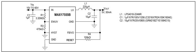
Figure 6. Fixed 5V, 50mA Step-Down Converter Output with 9.5V VINMIN
