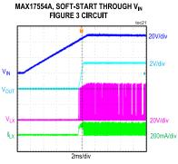
CONDITIONS: 3.3V OUTPUT, 66 Q LOAD,  $f_{SW}$  = 70kHz
