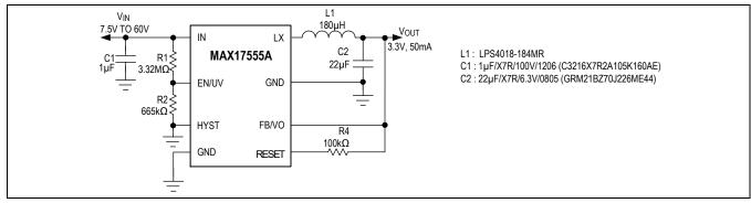
Figure 5. Fixed 3.3V, 50mA Step-Down Converter Output with 7.5V VINMIN
