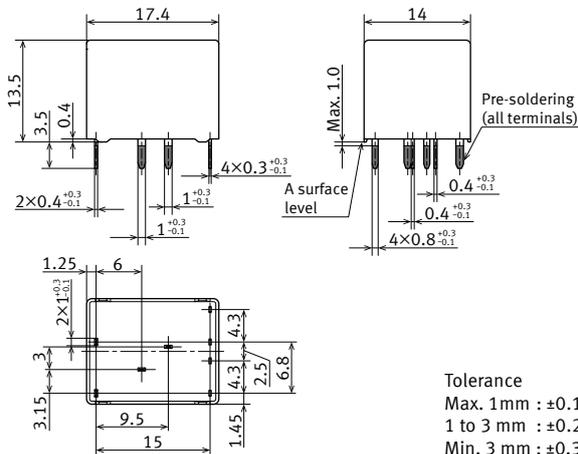
\* Dimensions (thickness and width) of terminal is measured after pre-soldering.
