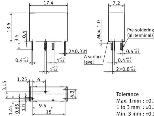
\* Dimensions (thickness and width) of is measured after pre-soldering. Intervals between terminals is measured at A surface level.
