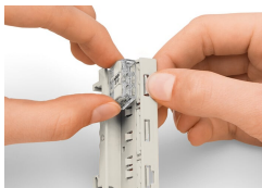
Removing a connector from the mounting carrier.
