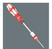
The screw gripper holds all screw profiles and sizes securely on the tool. Push the screw gripper onto the tip of the blade until the blade profile emerges from the rubber blade holder. Place the screw on the blade tip and fix it in the screw gripper. Pull the screw gripper further towards the handle until the two arms of the screw gripper rest on the screw head and are slightly spread.
