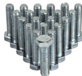
Hex Bolt 5/16-18 Length: 1-1/4" Use with T-Nut 6010 (p.237)
