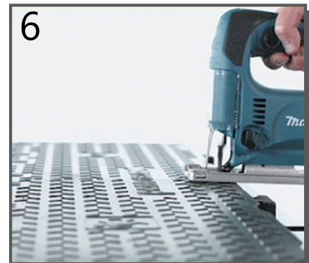
Cross 5 can even be cut into two using a compass saw. This allows you to create even more crossover structures.
