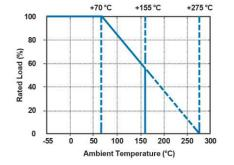
For resistors operated in ambient temperatures above 70°C, power rating must be derated in accordance with this curve.
