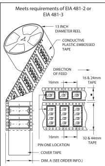
Each reel has a 15.750 inch (390 mm) minimum leader and a 6.30 inch (160 mm) minimum trailer.
