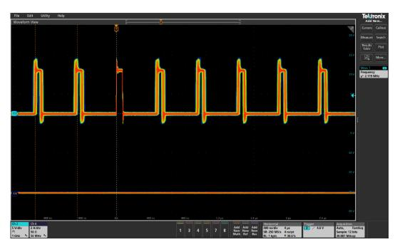
Figure 9 Sw at 0A (Ch2: Sw, Ch6: I<sub>o</sub>)
