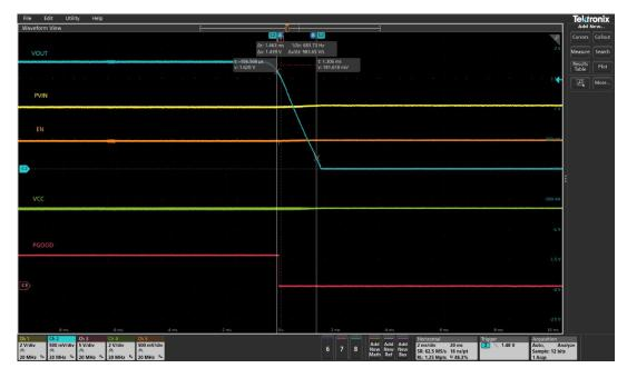
Figure 6 Soft turn off at 6A (Ch1:PVIN, Ch2: VOUT, Ch3: PG, Ch4:Vcc, Ch5: Enable)
