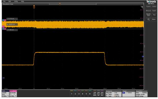
Figure 14 Transient response 3A to 6A (Ch6:I<sub>o</sub>, Ch7: V<sub>OUT</sub>), peak-peak deviation = 20.9mV
