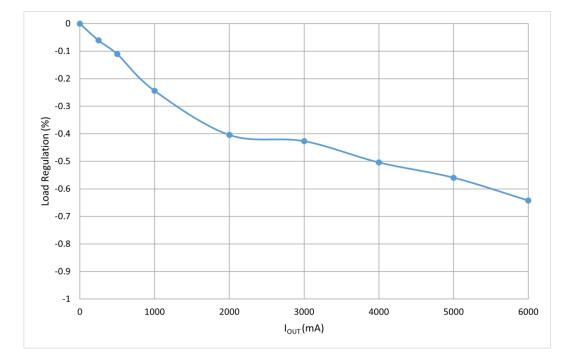
Figure 17 Load regulation ( $I_{0=}$  0–6A)
