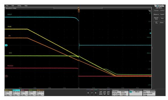
Figure 5 Shutdown with Enable de-assertion at 6A load (Ch1:PV<sub>IN</sub>, Ch2: V<sub>OUT</sub>, Ch3: PG, Ch4:V<sub>CC</sub>, Ch5: Enable)
