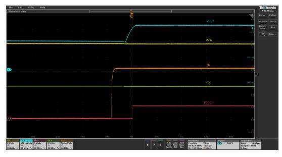
Figure 7 Startup into pre-bias (Ch1:PV<sub>IN</sub>, Ch2: V<sub>OUT</sub>, Ch3: PG, Ch4:V<sub>cc</sub>, Ch5: Enable)
