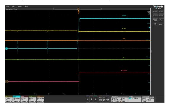
Figure 8 Over-current protection and auto-recover to 6A (Ch1:PV<sub>IN</sub>, Ch2: V<sub>OUT</sub>, Ch3: PG, Ch4:V<sub>CC</sub>, Ch5: Enable)
