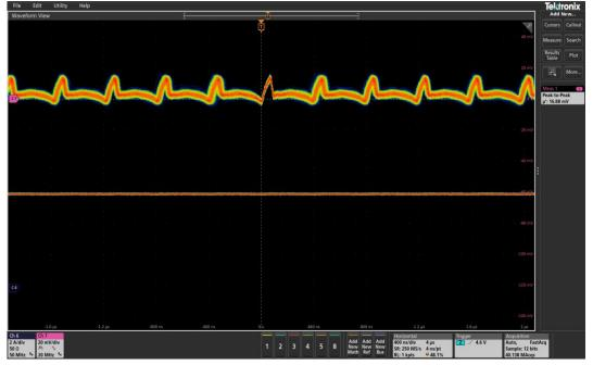
Figure 12 Vout ripple at 6A (Ch6:Io, Ch7:Vout), Peak-Peak Vout ripple = 16.9mV
