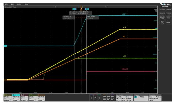
Figure 4 Startup with 6A load (Ch1:PV<sub>IN</sub>, Ch2: V<sub>OUT</sub>, Ch3: PG, Ch4:V<sub>CC</sub>, Ch5: Enable)
