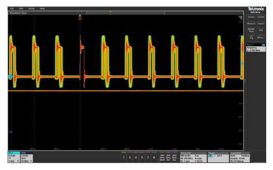
Figure 10 Sw at 6A (Ch2: Sw, Ch6: I<sub>o</sub>)
