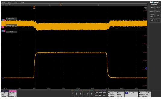
Figure 13 Transient response 0A to 6A (Ch6:I<sub>o</sub>, Ch7: V<sub>OUT</sub>), peak-peak deviation = 26mV
