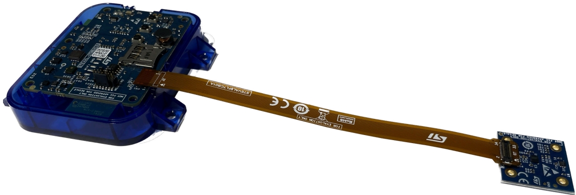
Figure 3. Plugging the flex cable onto the STWIN.box
