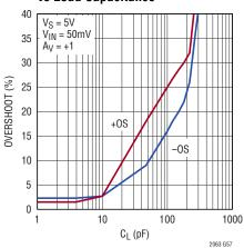
Small Signal Overshoot vs Load Capacitance
