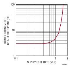
Figure 8. LTC2063 Power-Up Charge vs Supply Edge Rate
