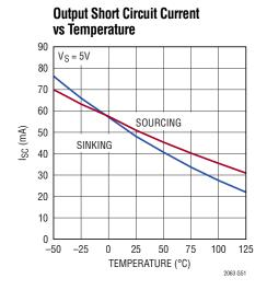
Output Short Circuit Current vs Temperature
