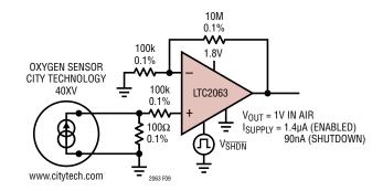
Figure 9. Micropower Precision Oxygen Sensor
