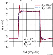
Small Signal Overshoot vs Load Capacitance
