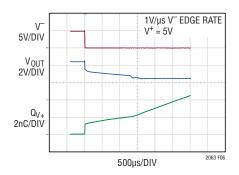
Figure 6. LTC2063 Charge Loss During Power-Up
