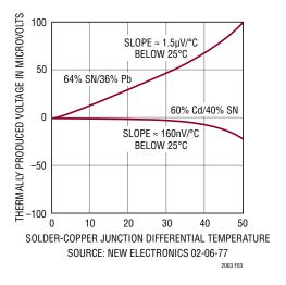
Figure 3. Solder-Copper Thermal EMFs
