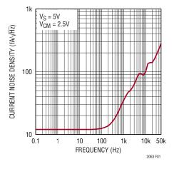
Figure 1. Input Current Noise Spectrum
