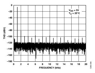
Figure 35. Total Harmonic Distortion (THD) at 1 kHz
