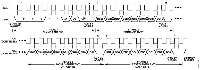
Figure 43. I<sup>2</sup>C Write Operation
