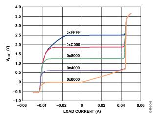
Figure 22. Source and Sink Capability at 3 V
