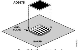
Figure 49. Pad Connection to Board
