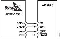
Figure 48. AD5675 to ADSP-BF531 Interface
