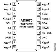
Figure 4. TSSOP Pin Configuration
