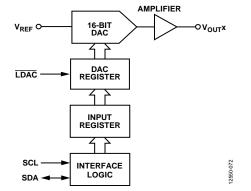
Figure 46. Simplified Diagram of Input Loading Circuitry for a Single DAC
