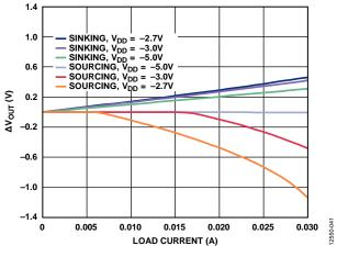
Figure 20. Headroom/Footroom (ΔVout) vs. Load Current
