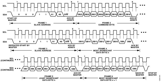
Figure 44. I<sup>2</sup>C Read Operation
