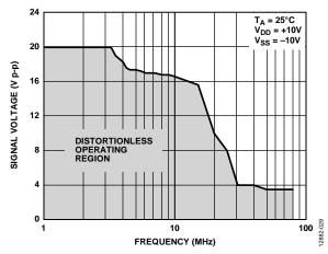
Figure 29. Large Signal Voltage Tracking vs. Frequency
