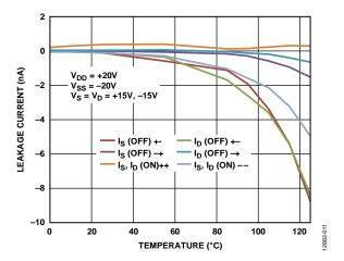
Figure 12. Leakage Current vs. Temperature, ±20 V Dual Supply
