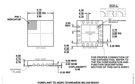
Figure 53. 16-Lead Lead Frame Chip Scale Package [LFCSP] 4 mm × 4 mm Body and 0.75 mm Package Height (CP-16-17) Dimensions shown in millimeters
