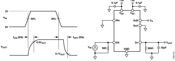
Figure 45. Enable Delay, ton (EN), toff (EN)
