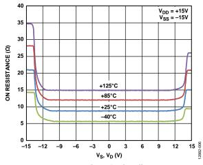
Figure 7.  $R_{ON}$  as a Function of  $V_5$  and  $V_D$  for Different Temperatures,  $\pm 15$  V Dual Supply
