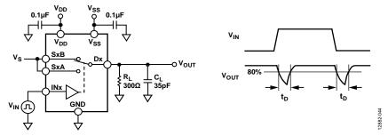
Figure 44. Break-Before-Make Time Delay,  $t_D$
