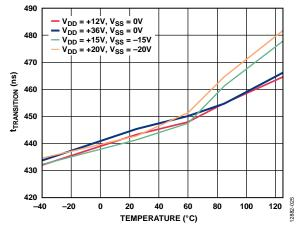
Figure 25. ttransition vs. Temperature
