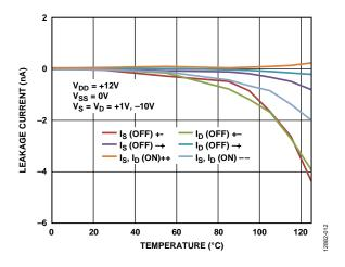
Figure 13. Leakage Current vs. Temperature, 12 V Single Supply
