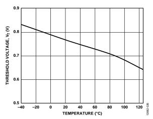
Figure 26. Threshold Voltage (V<sub>T</sub>) vs. Temperature
