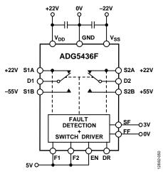
Figure 50. ADG5436F Under Example Overvoltage Conditions
