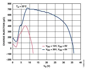
Figure 20. Charge Injection vs. Source Pin Voltage (Vs), Single Supply
