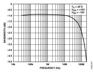
Figure 24. Bandwidth vs. Frequency
