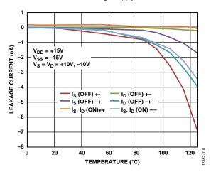
Figure 11. Leakage Current vs. Temperature, ±15 V Dual Supply
