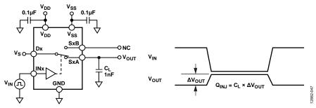
Figure 47. Charge Injection,  $Q_{\text{INJ}}$
