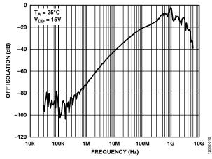
Figure 18. Off Isolation vs. Frequency
