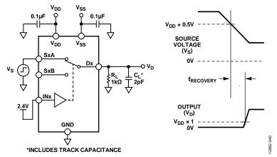
Figure 40. Overvoltage Recovery Time, trecovery
