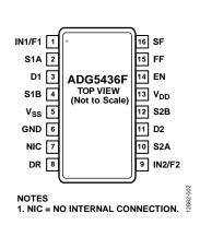
Figure 2. TSSOP Pin Configuration
