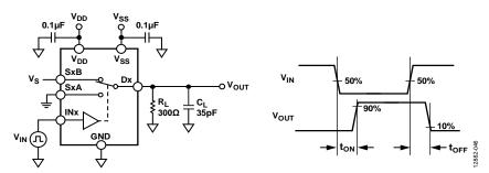
Figure 46. Address to Output Switching Times, ttransition
