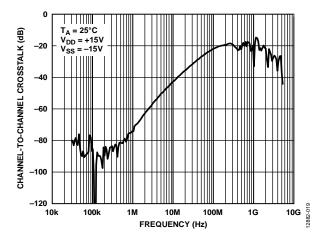
Figure 19. Channel-to-Channel Crosstalk vs. Frequency
