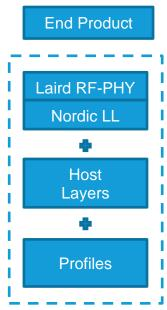
Figure 20: Scope of the qualification for an End Product Design
