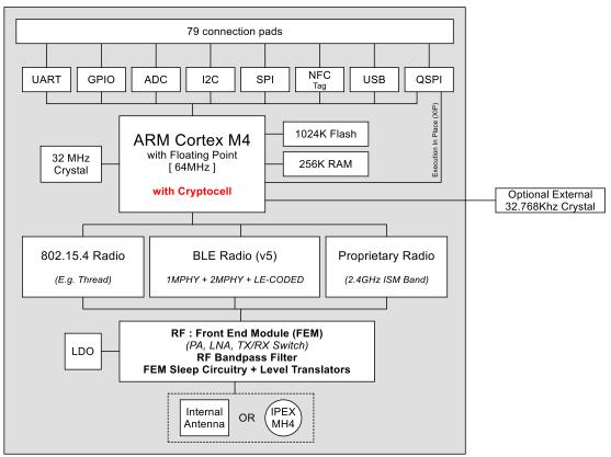
Figure 1: BL654PA block diagram
