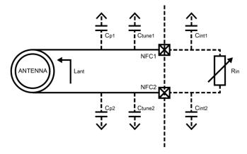
Figure 5: NFC antenna coil tuning capacitors
