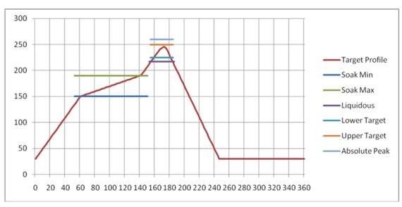
Figure 19: Recommended reflow temperature
