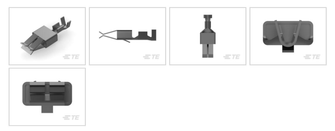
Terminal Type: Receptacle Mating Tab Width: 5.8 mm [.228 in ] Mating Tab Thickness: .8 mm [.031 in ] Terminal Transmits: 0–24 A (Low Power) Wire Size: 20–17 AWG
