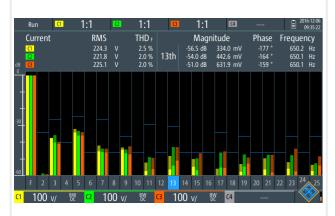
Harmonics analysis with magnitude, phase and frequency measurements for up to 64 harmonics and automatic limit testing.
