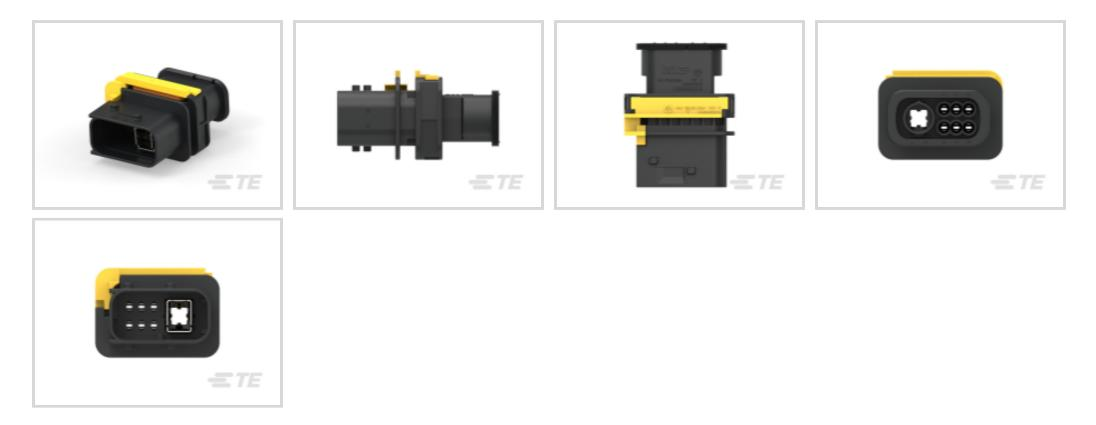
Connector & Housing Type: Housing for Male Terminals Mating Tab Width: .5 mm, 1.6 mm [ .019 in, .062 in ] Mating Tab Thickness: .4 mm, .6 mm [ .015 in, .023 in ] Connector & Keying Code: A Connector System: Wire-to-Wire
