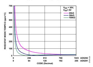
Figure 38. Rheostat Mode Tempco  $\Delta R_{WB}/\Delta T$  vs. Code
