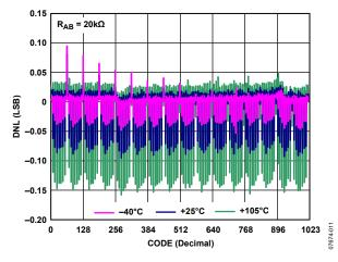
Figure 12. R-DNL in Normal Mode vs. Code vs. Temperature (AD5292)
