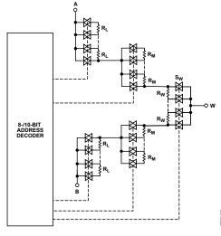
Figure 65. Simplified RDAC Circuit
