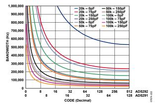
Figure 48. Bandwidth vs. Code vs Net Capacitance
