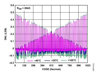
Figure 14. DNL in R-Perf Mode vs. Code vs. Temperature (AD5292)
