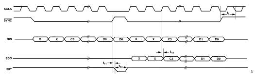
Figure 4. Read Timing Diagram, CPOL = 0, CPHA = 1
