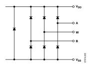
Figure 69. Maximum Terminal Voltages Set by V<sub>DD</sub> and V<sub>SS</sub>
