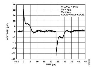
Figure 53. Digital Feedthrough
