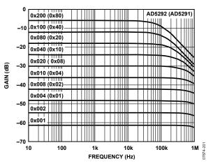
Figure 45. 100 kΩ Gain vs. Frequency vs. Code
