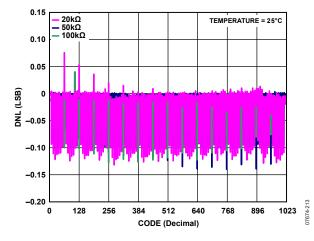
Figure 15. R-DNL in Normal Mode vs. Code vs. Nominal Resistance (AD5292)
