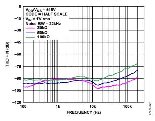
Figure 44. THD + Noise vs. Frequency
