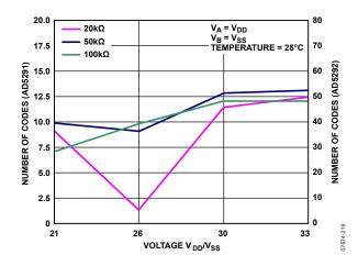
Figure 57. Code Range > 1% R-Tolerance Error vs. Voltage
