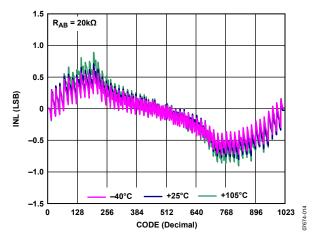
Figure 13. INL in R-Perf Mode vs. Code vs. Temperature (AD5292)
