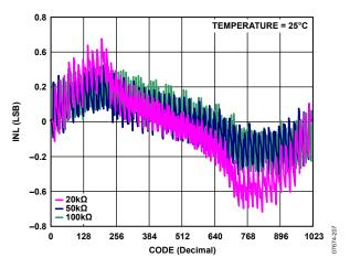
Figure 16. INL in R-Perf Mode vs. Code vs. Nominal Resistance (AD5292)
