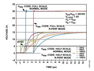
Figure 50. 20 kΩ Large-Signal Settling Time from Code Zero Scale
