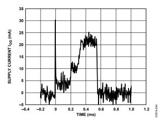
Figure 49. IDD Waveform While Blowing/Reading Fuse
