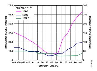
Figure 56. Code Range > 1% R-Tolerance Error vs. Temperature
