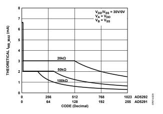
Figure 51. Theoretical Maximum Current vs. Code
