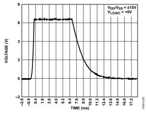
Figure 55. V<sub>EXT CAP</sub> Waveform While Writing Fuse
