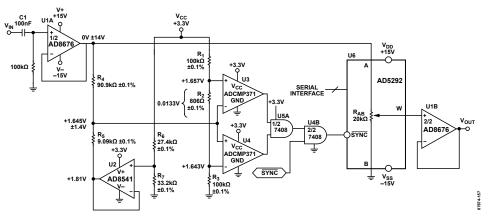
Figure 74. Audio Volume Control with Zipper Noise Reduction
