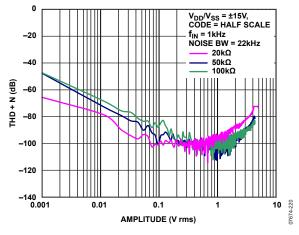
Figure 47. THD + Noise vs. Amplitude
