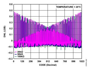
Figure 17. DNL in R-Perf Mode vs. Code vs. Nominal Resistance (AD5292)
