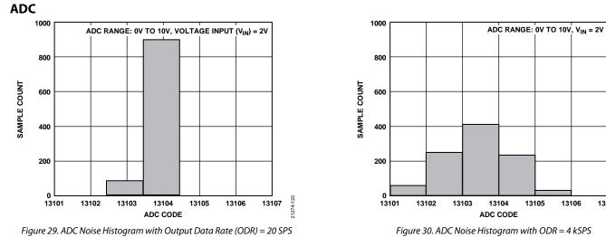
Figure 30. ADC Noise Histogram with ODR = 4 kSPS
