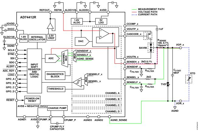
Figure 41. Resistance Measurement Configuration
