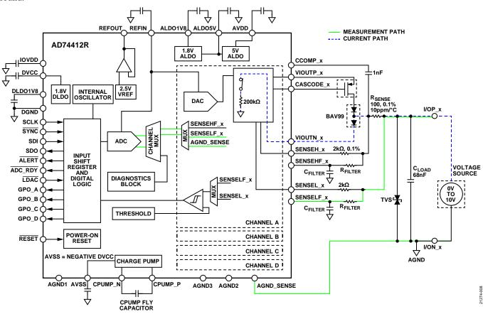
Figure 37. Voltage Input Mode Configuration
