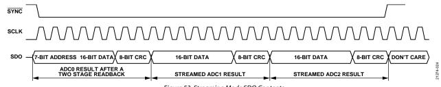
Figure 53. Streaming Mode SDO Contents
