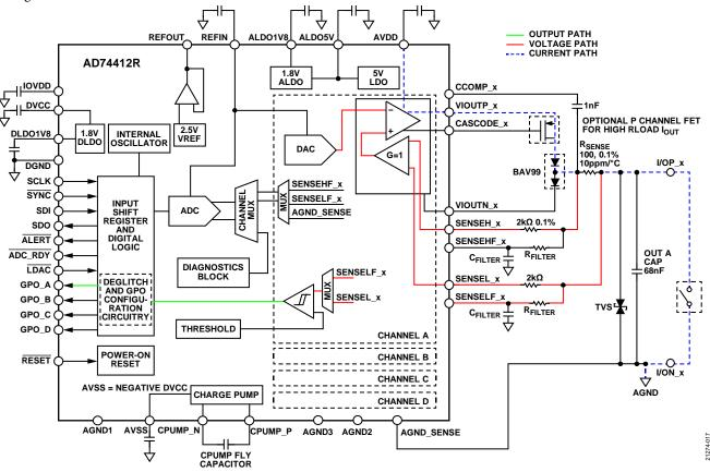
Figure 46. Digital Input, Loop Powered Configuration Mode
