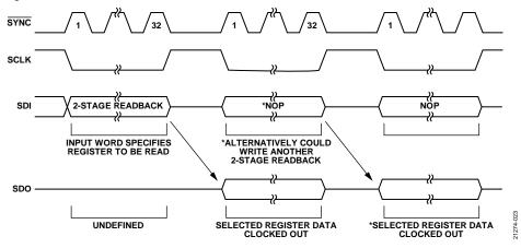
Figure 52. Two-Stage Readback Timing Diagram
