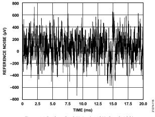
Figure 26. Peak-to-Peak Noise (100 kHz Bandwidth)
