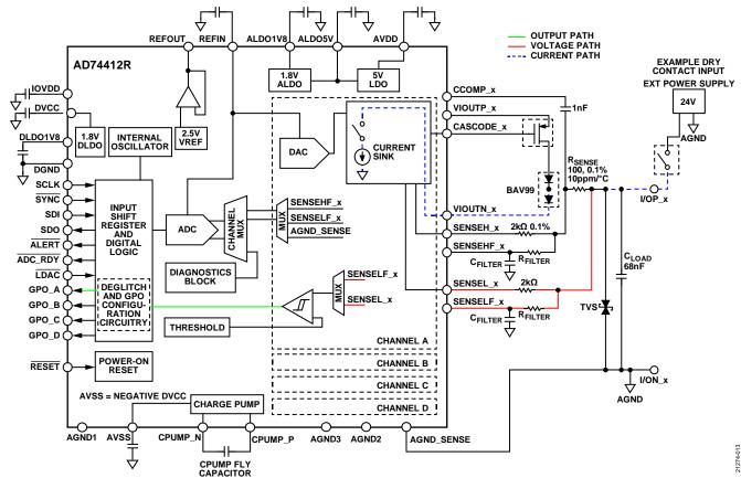
Figure 42. Digital Input Logic Mode Configuration
