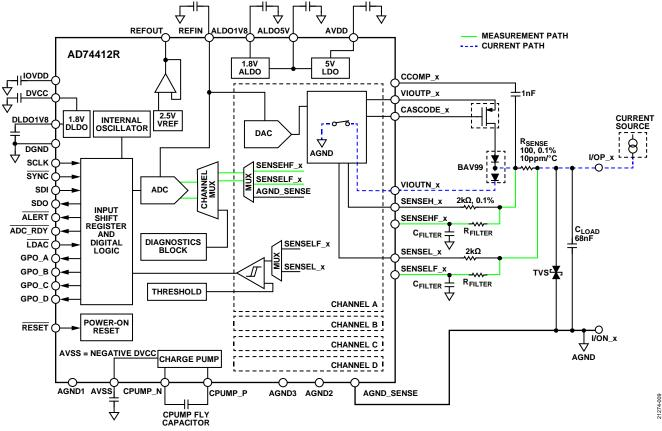
Figure 38. Current Input, Externally Powered Mode Configuration
