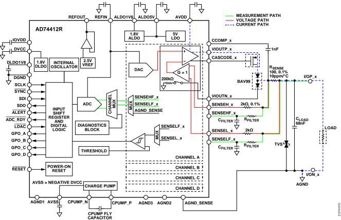
Figure 39. Current Input, Loop Powered Mode Configuration
