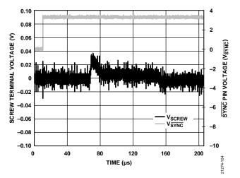
Figure 8. Screw Terminal Voltage (V<sub>SCREW</sub>) vs. Time on Voltage Output Enable
