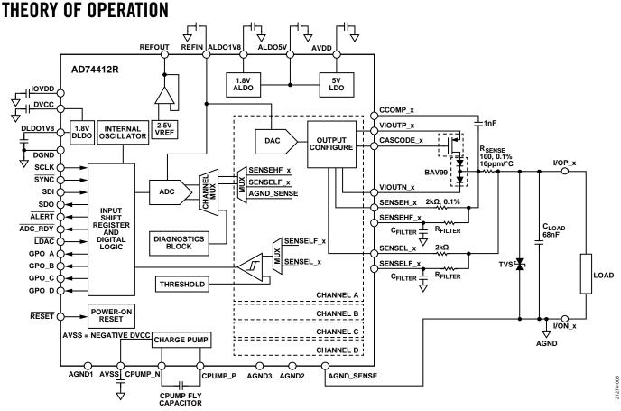
Figure 34. Detailed Functional Block Diagram
