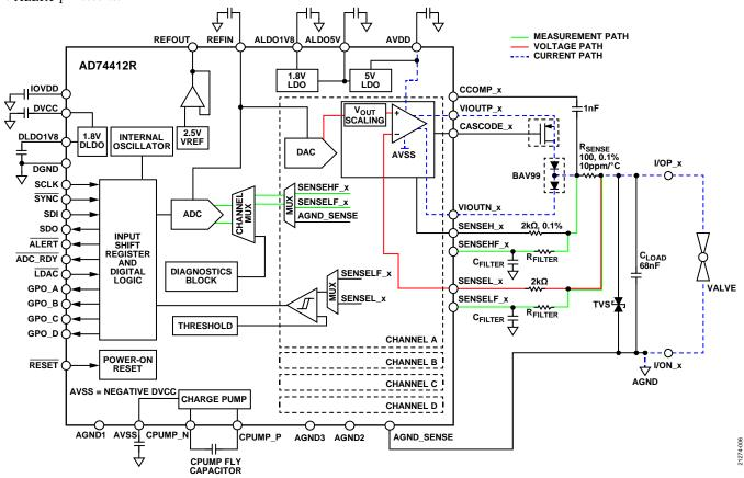
Figure 35. Voltage Output Mode Configuration
