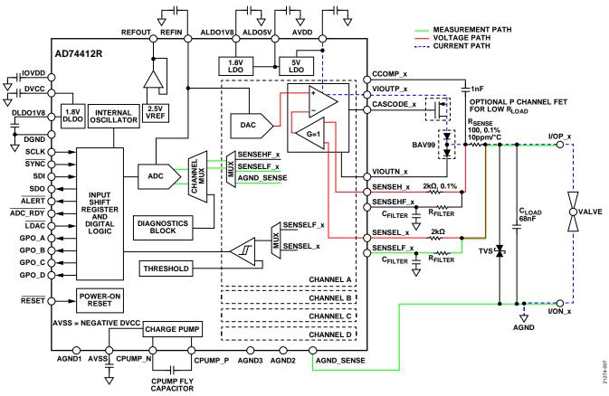
Figure 36. Current Output Mode Configuration
