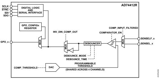
Figure 45. Digital Input Configuration
