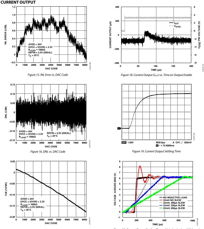
Figure 20. Current Output Settling Time with Inductive Load With and Without Slew Rate Enabled
