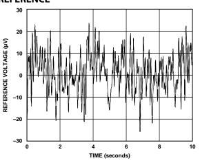
Figure 25. Peak-to-Peak Noise (0.1 Hz to 10 Hz Bandwidth)
