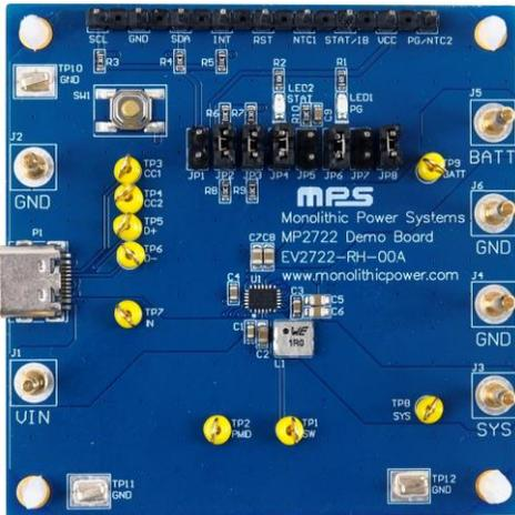
Figure 2: EV2722-RH-00A Evaluation Board
