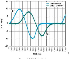
Figure 4. DAC Output Latency
