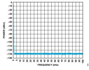
Figure 5. CN0584 Analog Input Acquisition Spectrum
