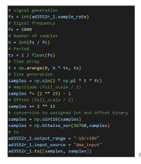
Figure 10. Example DAC Output Generation with Python
