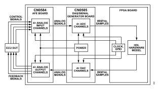
Figure 2. Hardware-in-the-Loop Simulation Setup
