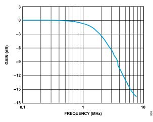
Figure 9. DAC Output Frequency Response
