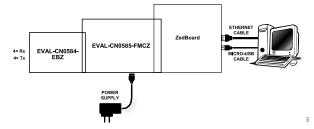
Figure 13. CN0584 Functional Test Block Diagram
