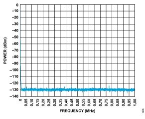
Figure 6. Analog Input Acquisition Spectrum to 1 MHz
