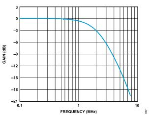
Figure 8. ADC and DAC Filter Composite Response
