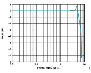
Figure 7. ADC Input Frequency Response
