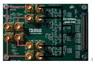
Figure 14. AFE Board I/O Setup
