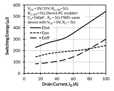
Figure 19. Clamped inductive switching energy vs. drain current at  $V_{DS}$  = 400V and  $T_J$  = 25°C
