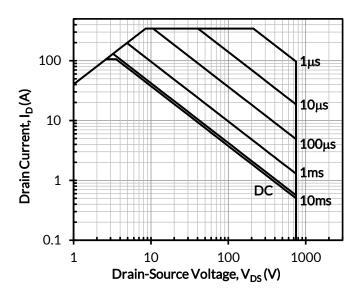
Figure 17. Safe operation area at  $T_C$  = 25°C, D = 0, Parameter  $t_D$
