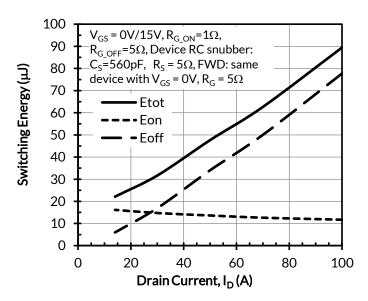
Figure 20. RC snubber energy loss vs. drain current at  $V_{DS}$  = 400V and  $T_J$  = 25°C
