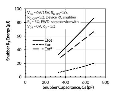
Figure 23. Clamped inductive switching energy vs. Snubber Capacitance Cs at  $V_{DS} = 400V$ ,  $I_D = 70A$ , and  $T_J$ = 25°C
