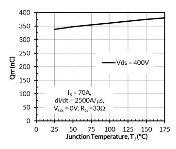
Figure 18. Reverse recovery charge Qrr vs. junction temperature
