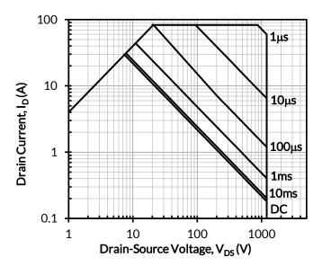
Figure 17. Safe operation area at  $T_C$  = 25°C, D = 0, Parameter  $t_p$
