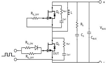
Figure 23. Schematic of the half-bridge mode switching test circuit with device RC snubbers ( $R_{s1}$  = 10 $\Omega$ ,  $C_{s1}$  = 95pF) and a bus RC snubber ( $R_{S}$  = 2.5 $\Omega$ ,  $C_{S}$ =100nF).
