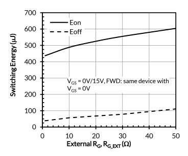
Figure 20. Clamped inductive switching energies vs.  $R_{G,EXT}$  at  $V_{DS}$  = 800V,  $I_D$  =20A, and  $T_J$  = 25°C
