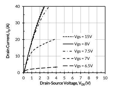
Figure 1. Typical output characteristics at  $T_J$  = - 55°C, tp < 250 $\mu$ s
