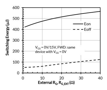
Figure 20. Clamped inductive switching energies vs.  $R_{G,EXT}$  at  $V_{DS}$  = 800V,  $I_D$  =25A, and  $T_J$  = 25°C
