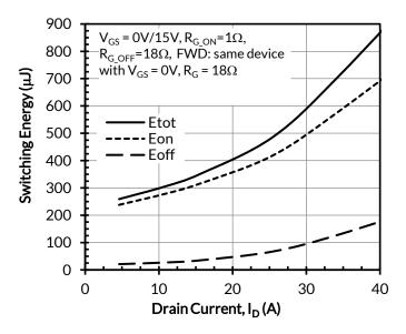
Figure 19. Clamped inductive switching energy vs. drain current at  $V_{DS}$  =800V and  $T_J$  = 25°C
