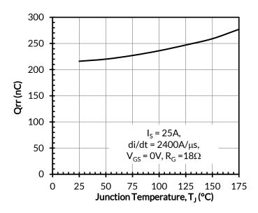
Figure 18. Reverse recovery charge Qrr vs. junction temperature at  $V_{DS}$  = 800V
