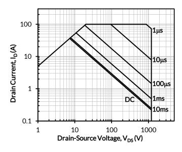
Figure 17. Safe operation area at  $T_C$  = 25°C, D = 0, Parameter  $t_p$
