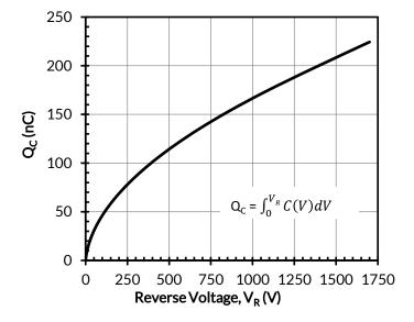
Figure 8. Typical capacitive charge vs. reverse voltage
