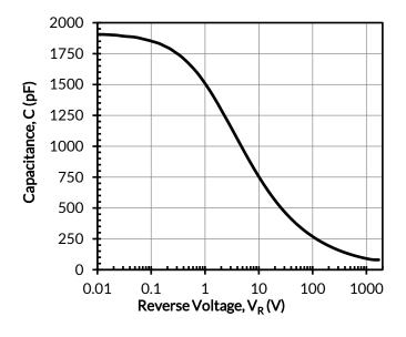
Figure 7. Capacitance vs. reverse voltage at 1MHz
