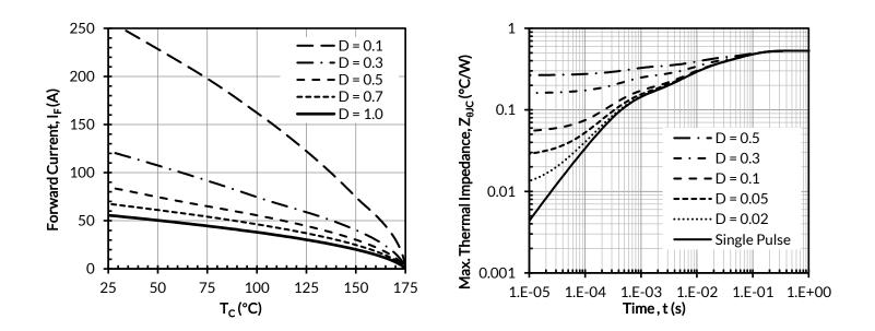
Figure 5. Diode forward current
