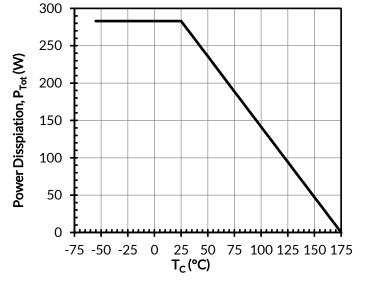
Figure 4. Power dissipation
