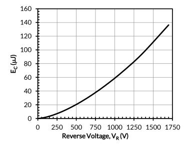
Figure 9. Typical capacitance stored energy vs. reverse voltage
