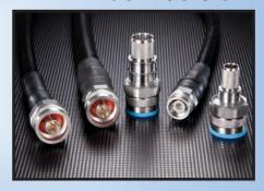
An extensive selection of LMR® connectors with crimp or clamp outer conductor attachment, and solder or non-solder 'EZ' center pins are available, *including* the new X series which does not require braid trimming. All common interfaces are available. Times'  $Advantage^{TM}$  series connectors are well known for their quality and reliability.
