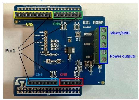
Figure 2. Evaluation board connections
